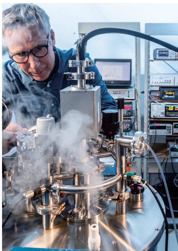
Implementation of the BIPM quantum Hall resistance for the realization of the electrical resistance unit (ohm) based on the Planck constant and the elementary charge, two foundational constants of the International System of Units (SI).
